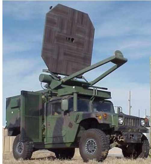
Active Denial System Advanced Concept Technology Demonstration System 1
